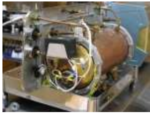
The completed machine without the main body. The two free-floating wires connect to the fluorescent light on the main body.
