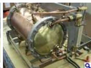
Final fitting of the sight glass and other pipes.
