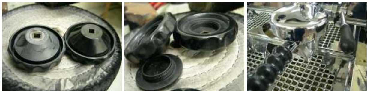
Repolishing the original Bakelite proved tricky but worthwhile. Steam valve knobs before left and after right.
