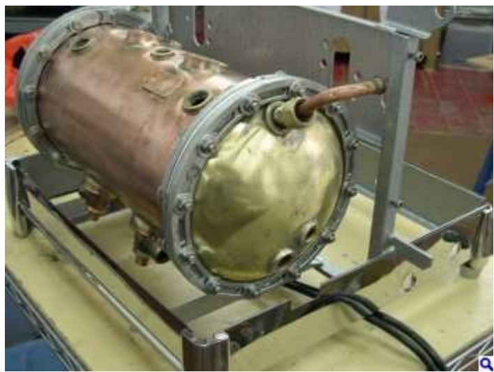
The rebuilt boiler being test-fitted onto the frame.
