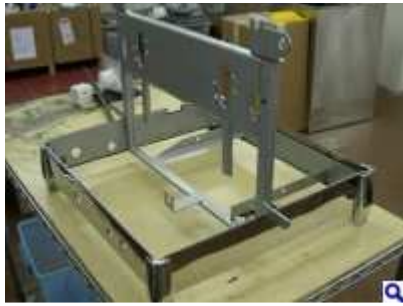
Repainted frame with bottom steel panels on.
